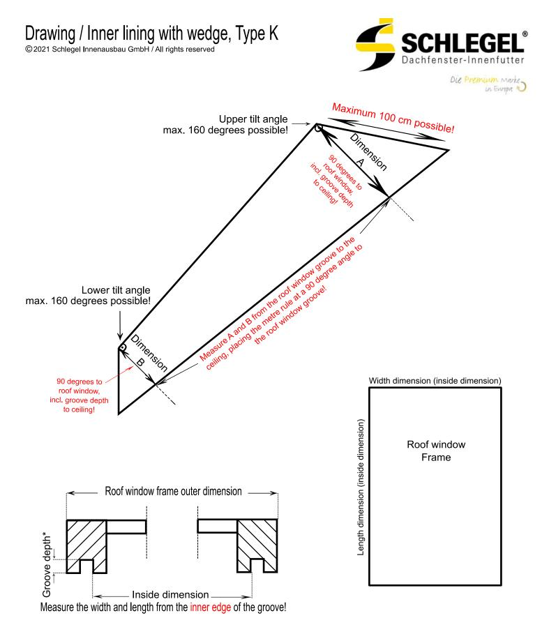
\*Groove depth: To compensate for unevenness on the ceiling, subtract approx. 4 mm in the groove from the total lining depth!
