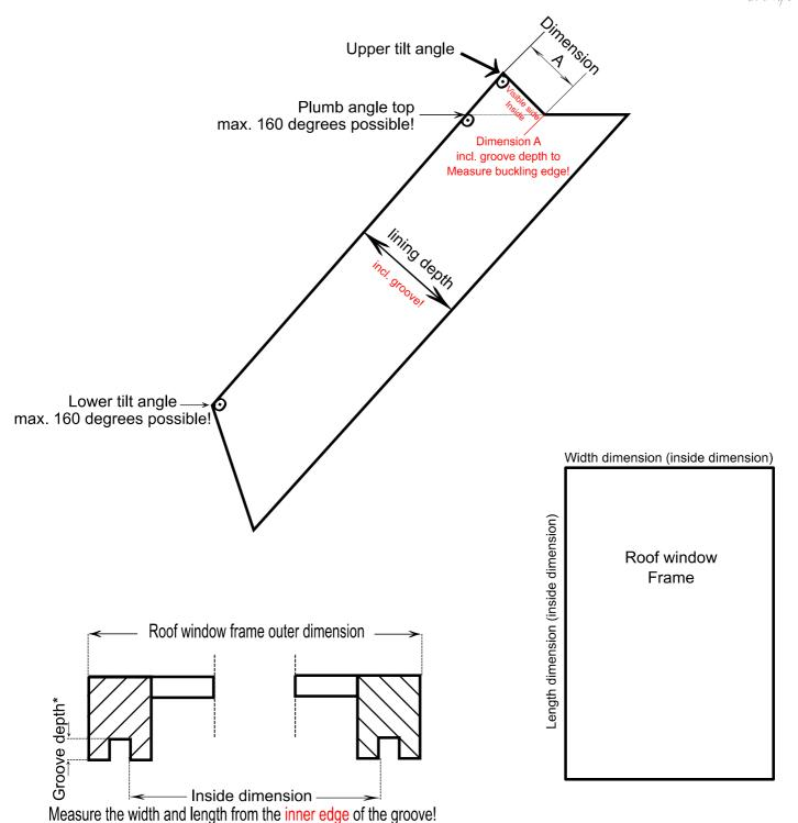
\*Groove depth: To compensate for unevenness on the ceiling, subtract approx. 4 mm in the groove from the total lining depth!
