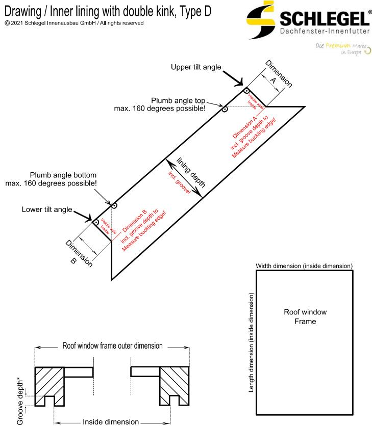
Measure the width and length from the inner edge of the groove!
