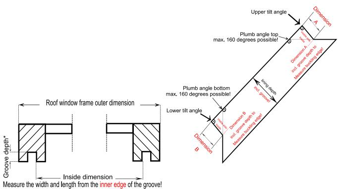
\*Groove depth: To compensate for unevenness on the ceiling, subtract approx. 4 mm in the groove from the total lining depth!
