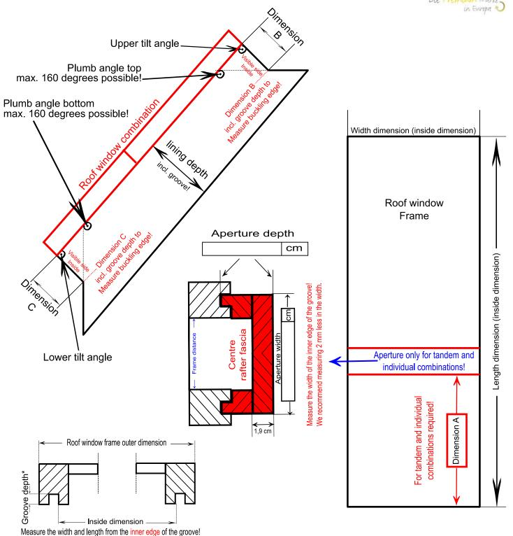
measure the which and length from the line edge of the groove:
