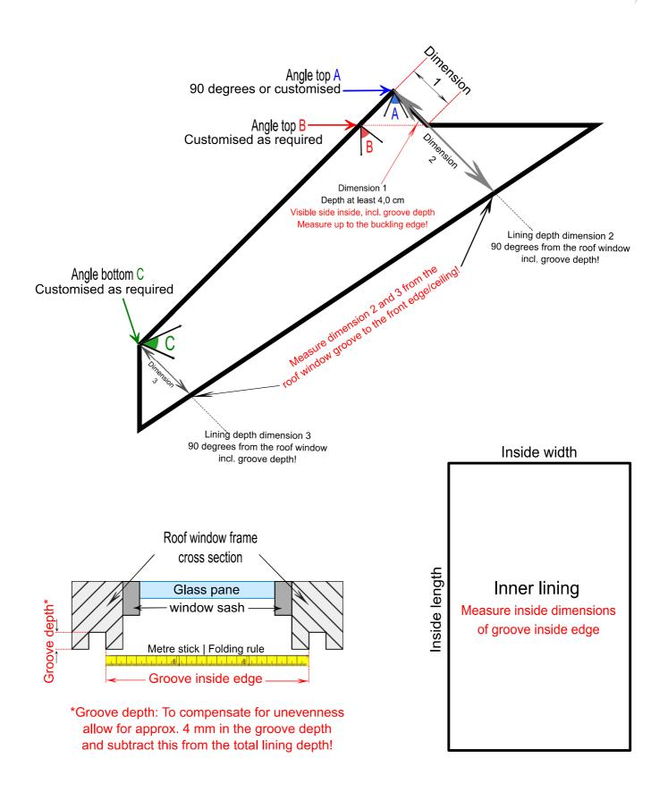
Please note, our inner linings have a material thickness of 19 mm. Make vapour barrier with sufficient clearance for the inner lining!
