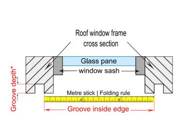
\*Groove depth: To compensate for unevenness allow for approx. 4 mm in the groove depth and subtract this from the total lining depth!
