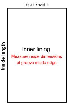
Please note, our inner linings have a material thickness of 19 mm. Make vapour barrier with sufficient clearance for the inner lining!
