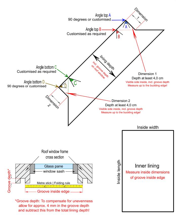
Please note, our inner linings have a material thickness of 19 mm. Make vapour barrier with sufficient clearance for the inner lining!
