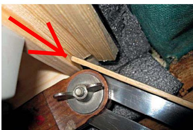
Lay the metre rule in the groove to simulate the lining, then measure the angle.
