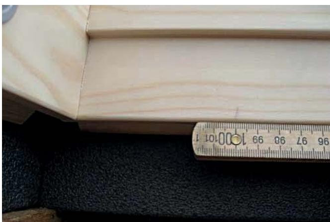
Measure the width to the inside edge of the opposite groove (inside dimension).
